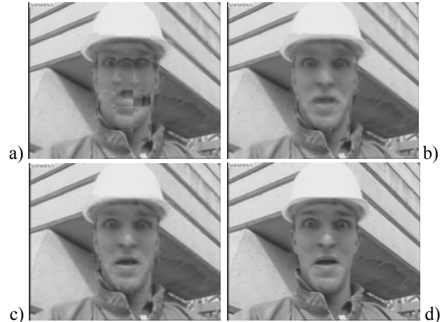
Figure 4 Frame 93: a) MCTI b) MCTI with the 3D model rendered on top c) decoded picture (MCTI + model + parity bits) d) original picture
